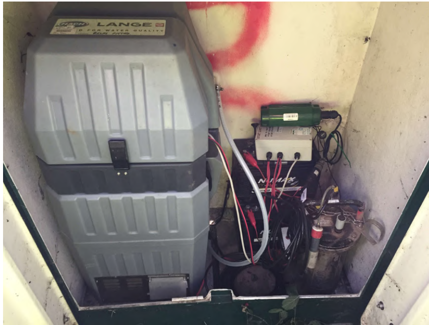
Figure 2.3: Flow and quality monitoring device used for data collection.
